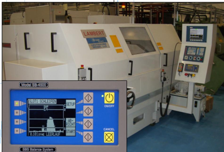
Diameter (OD), Inside Diameter (ID) and Track and Lip (Vector) grinding of roller bearings from 50mm to 450mm diameter. The machine has a point wheel dresser unit as standard, but has also been retrofitted with a custom made radius dressing attachment, capable of generating 'Gothic Arch' wheel profiles. The machine was originally fitted with a
