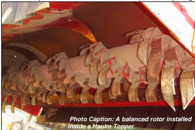
Photo Caption: A balanced rotor installed inside a Haulm Topper
